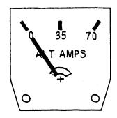
AMMETER THAT HAS NOT BEEN CALIBRATED.
